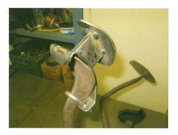
The extender slips over the existing reverse pedal and is secured by a small U-bolt. The pedal section is made from 3 mm flat bar shaped similar to the actual pedal to allow the after-market pedal rubber to be used again. The slotted section fitting snugly over the pedal is made from 40 mm flat bar of 2 mm thickness. The two sections are connected using a piece of 40 mm flat bar of 8 mm thickness and the actual throw achieved is 38 mm.
